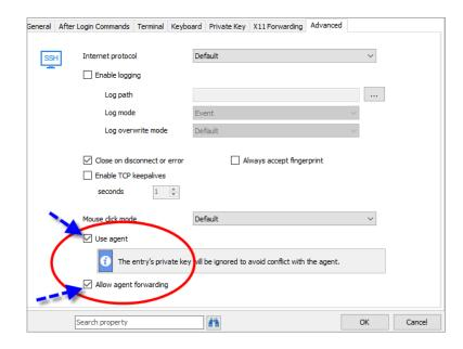
For example, once you've SSHed into a machine, it will continue to SSH from it to the next machine, using the same key. I'm sure you can see how useful this can be when comes time to deploy to a server! It will allow you to use your local SSH keys instead of having to leave them hanging on your server without any passphrase protecting them.
